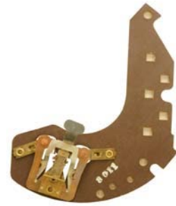
reversing switch mounting holes : 1-1/4 & 3-9/16 c.-c.
