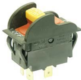
on-off safety switch removable lock, 4 terminals 20A @ 125-277VAC 1hp rating
