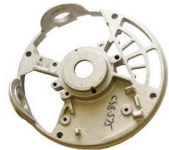
switch end bell, open, brg size 6203 threaded conduit hole
